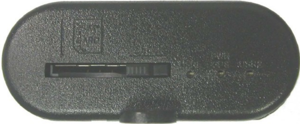
Figure 1: Front View of the GPS-206. Note the SIM Card Access.
