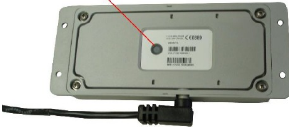
Figure 6: Bottom view of the GPS-207DC
