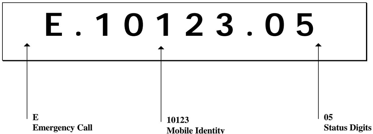
The ARi-195e can decode up to 99 different status's which are then displayed on the right hand side of the console. To further assist the dispatcher, "emergency" calls and "request to talk" calls (also called autoCALL) have an associated Alpha character, E and A respectively, which are also displayed when the appropriate sequence is received from a mobile. A separate "alert tone" is generated for the three types of calls, Emergency, AutoCALL and Normal calls.
