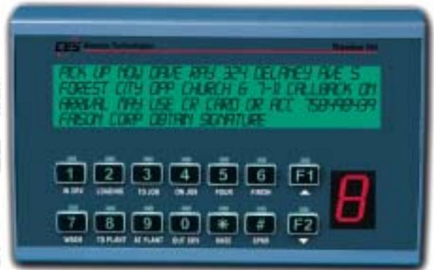
The TRK-240 is an advanced mobile data display and status terminal featuring intelligent messaging capabilities that works with your existing mobile radio system. Featuring a backlit 4 x 40 display together with 14 "real" backlit user programmable silicone rubber keys, the TRK-240 is loaded with a host of advanced features. The unit is enclosed in a rugged "industrial" enclosure and sealed from dust and the harsh environment into which these devices are often installed.
